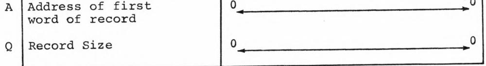
If logical record processing has been specified, the address in the high order half of the A-register is the current record index. In physical record processing, the address is that of the first word of the tape block.
